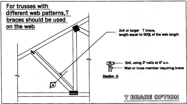
This information is intended to illustrate certain options for transferring web buckling forces to the roof diaphragm in pitched and parallel chord trusses. It is intended to provide typical configurations only. These configurations are deemed to be relatively conservative, however will not cover all cases. Qualified persons must ensure specific applications will resist imposed loads.
